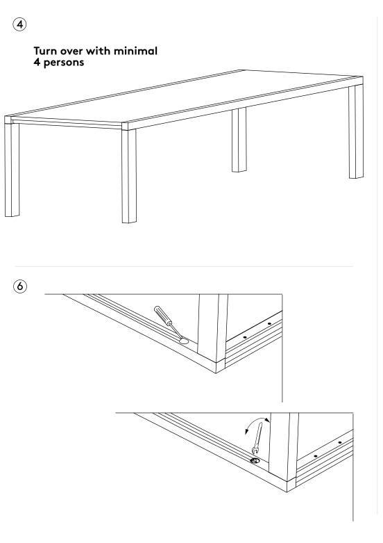
Instructions to correct the evenness of the table-top. Can be corrected on two sides by means of tightening the sludge. As a result of thightening this sludge, the table-top will "swell" a little.
